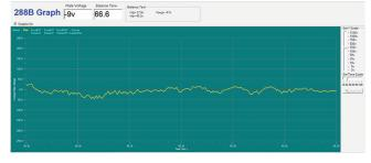
· Induction Switching Voltage from Pulsed AC Ionizer · Peak-to-Peak value: +305V to - 393V.
